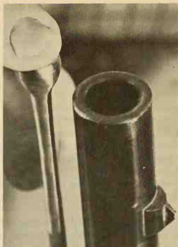
In returning the ramrod to its seat in the stock, use the tip of a finger so as to keep all parts of the hand clear of the bullet's path in the event of an accidental discharge.
