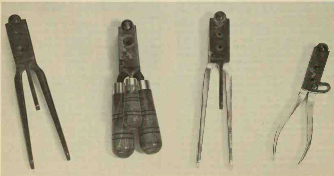
A variety of old-style molds as they are produced today in replica form by, oddly enough, Replica Arms. Those with plain, short metal handles become impossible to use after
