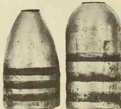
Lyman #575213 minie is of traditional shape with deep conical base hollow, weighs 460 grains. Right is new #57730, 570 grains, with larger cylindrical base cavity, and a good bit more bearing surface for more accurate alignment in bore during ramming and seating.
