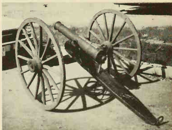
Dixie Civil War Field Cannon with 43-inch tube and 2-3/16-inch bore. Mounted on a semi-modern carriage consisting of a welded trail and cheeks and old wood wagon wheels. It's quite popular among cannon buffs.
