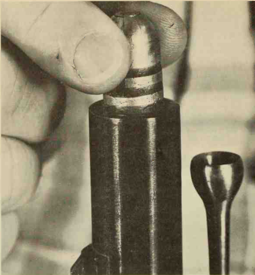
Properly greased minie bullet (Lyman's new #57730, weighing 570 grains, here) should be started straight and as far into the muzzle as possible with the fingers. Note that no part hand is actually directly over the muzzle.
