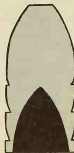
Typical Minie bullet with its large base hollow which causes the bullet to be expanded by powder gases to engage the rifling, while still being small enough for easy loading through the muzzle.
