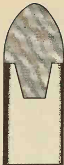
Swaged bullets may be solid or two-piece as is this one intended for a slug gun. Nose portion is hard to resist deformation during ramming, body soft to take the rifling easily.
