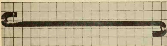
One of the simplest forms of breech plug wrench is this. A bar of steel is simply forged around a form, and then filed to fit the tang closely. A close fit is necessary to avoid damage to the plug. With torch, hammer and anvil you can make one of these in 20 minutes. They are available ready-made from Dixie Gun Works.
