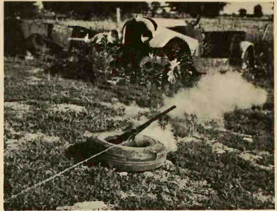
The cheapest and simplest method of tying a gun down for proof-firing is to place it in an old auto tire like this; then fire by means of a long cord or wire tied to the trigger. This old 12-bore double took the heavy charge in stride.
