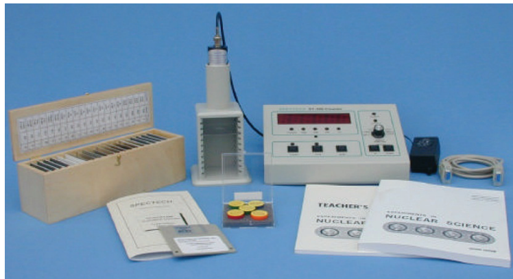
Figure 3: ST-350 Counter with GM Tube and stand (Counter box, power supply – transformer, GM Tube, shelf stand, serial cable, and a source holder for the stand) from Spectrum Techniques (USA).
