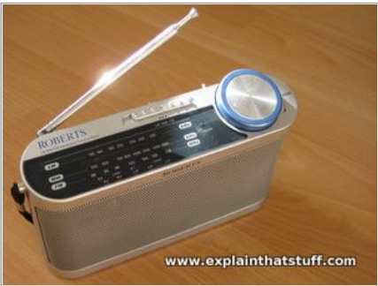
Photo: This is a typical one-way radio: it will receive things like music broadcasts from radio stations, but it can't transmit. A walkie-talkie can send and receive, so it's called a two-way radio.
